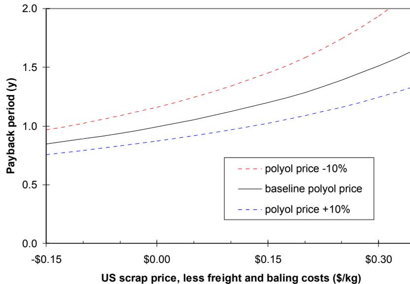
Picture 6 - Sensitivity plot showing variation of the cost savings with scrap-foam value and Polyol price at a level of 10% powder in a conventional slabstock foam (25 kg/m<sup>3</sup>, 150 N).
