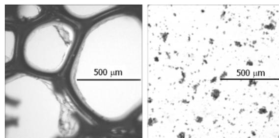
Picture 4 - Photomicrographs of the cell structure of a flexible foam and Powdered Urethane
