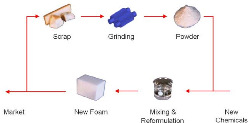
Picture 3 – Recycling Process: from the scrap to new flexible foam
