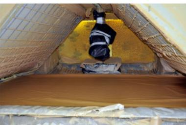
The spray head ensures a perfect mix and deposition of the liquid blend, while the closed loop control system of the Cannon B2 dosing machine keeps all the variables (temperature, viscosity, mixing ratio, recirculation), within the desired working range.
