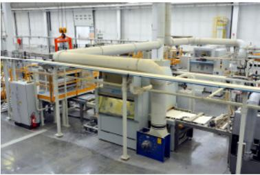
Two complete composite lines are installed side by side in this factory: the simplest features one Cannon dispensing station, while the more complex one features two Cannon stations. These are used in sequence, one after the other, when a double or a triple laminate is produced.
