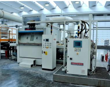
The entirely automated Composite line is used for applying the glass fiber mat on the slab to improve LAMINA sturdiness, lightness and elasticity.
