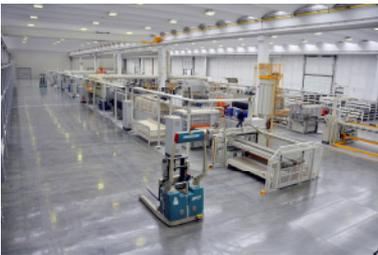
A single line can manufacture 70 standard slabs per hour, while the more complex one can produce up to 35 double and triple slabs per hour.
