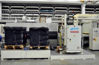
The slabs are then passed into an horizontal electric heater to stabilise the temperature (37 °C – 40 °C) of the material to be processed; and finally they are rotated by 180° and centred. With the rough face up, they enter in the spraying cabin. (Picture 11)
