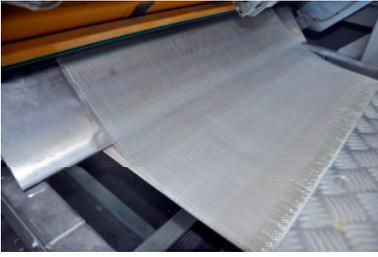
After the application of the adhesive the slabs go to the glass fiber application area, where a precisely cut-to-size piece of bi-directionally oriented glass fiber mat, is simply laid over the rigid support. (Picture 14)
