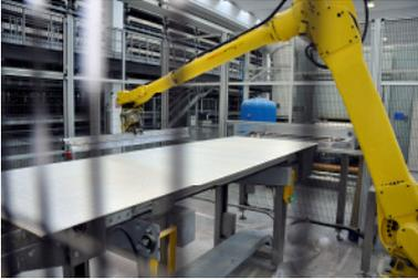
The station is equipped with an automatic tool-change system, so that the operator can change the squeegee without stopping the working cycle. (Picture 15)
